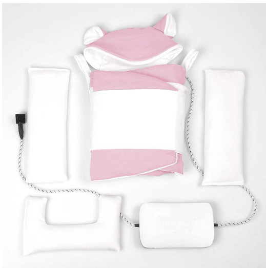
Figure 1 Hugsy comfort set prototype. Hugsy swaddling blanket (in center), side-positioning pillows (left and right side), foot positioning pillow (bottom left), Hugsy heartbeat recording and playback module (bottom right).
