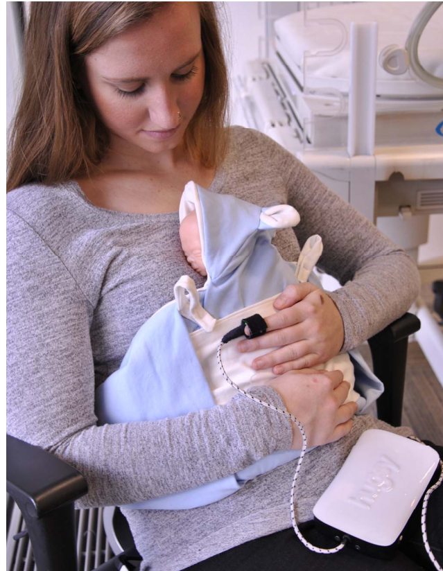
Figure 2 Hugsy use case simulation. Mother performing kangaroo care wearing Hugsy blanket, while recording heartbeat using heartbeat module.
